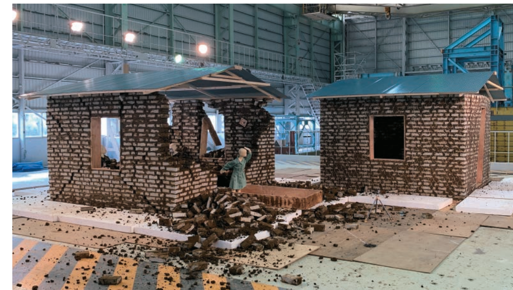
Confirming effectiveness of jacketing method using Large-scale Earthquake Simulator (photo: joint research by NIED/Chiba University and others)
